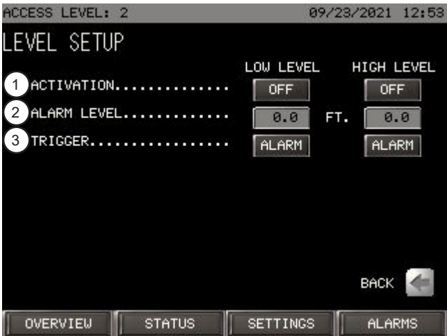
1. Activation - Activate or disable the low level and high level alarm input. 2. Alarm level - Enter the levels at which the low level and high level alarms occur. 3. Trigger - Select whether to trigger an alarm or a fault.
